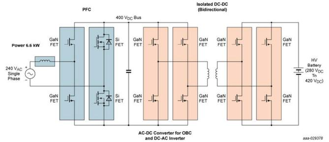
Figure 5 AC-DC PFC stage and isolated DC-DC configuration
