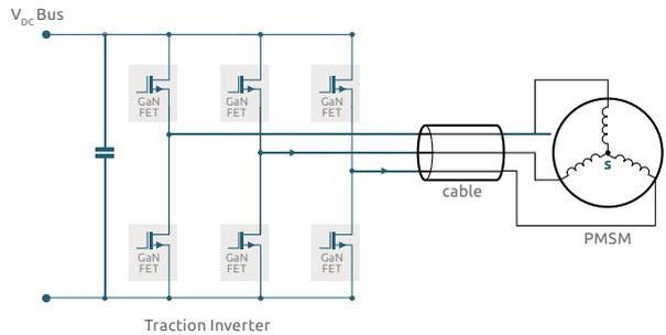
Figure 6 Traction Inverter
