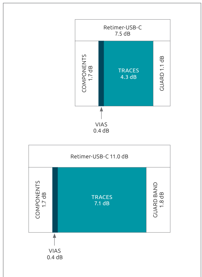
Fig. 4: Composition of host insertion loss budgets, USB4 specification vs. Kandou capability
