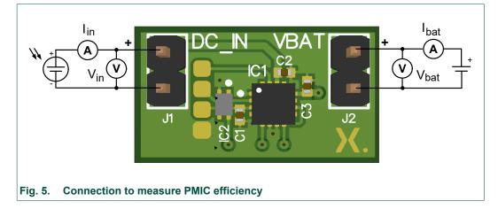
The efficiency of the PMIC can be calculated using the formula below:
