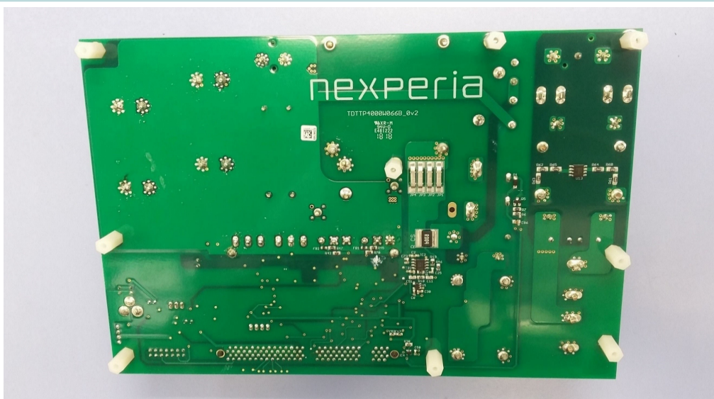
Fig. 3. 4 kW Totem-pole PFC evaluation board; bottom side
