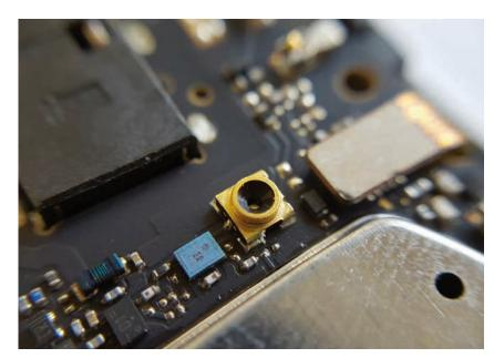
Figure 102 | Internal antenna contacts
