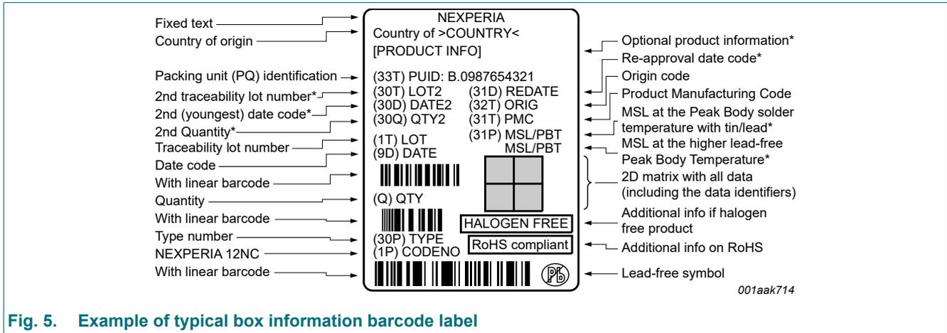
Fig. 5. Example of typical box information barcode label
