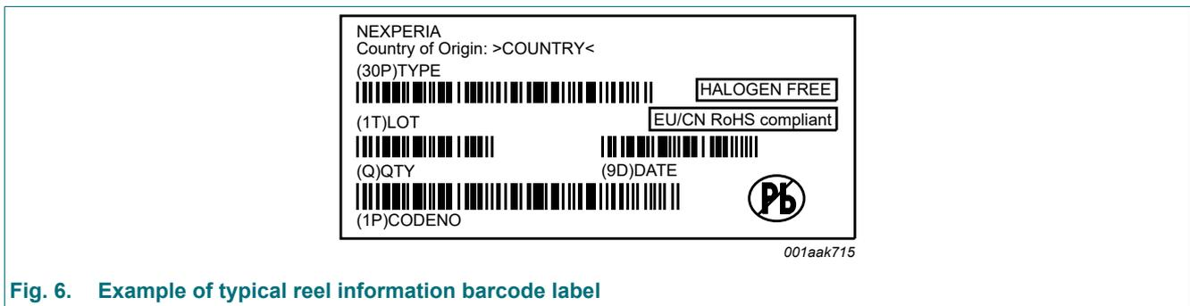
Fig. 6. Example of typical reel information barcode label
