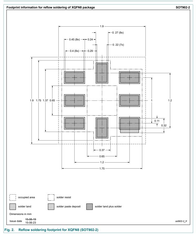
plastic, leadless extremely thin quad flat package; 8 terminals; 0.5 mm pitch; 1.6 mm x 1.6 mm x 0.5 mm body
