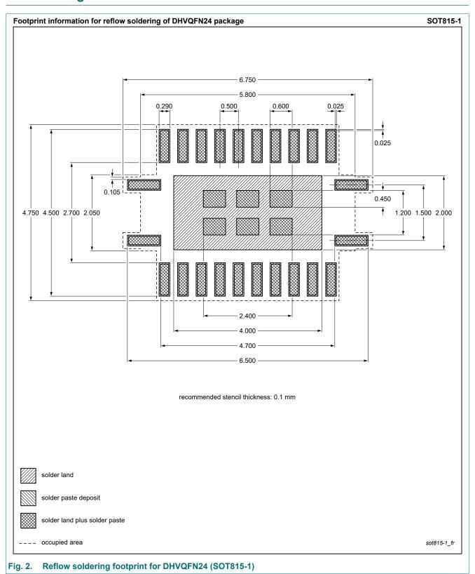
plastic, leadless dual in-line compatible thermal enhanced very thin quad flat package; 24 terminals; 0.5 mm pitch; 5.5 mm x 3.5 mm x 1 mm body
