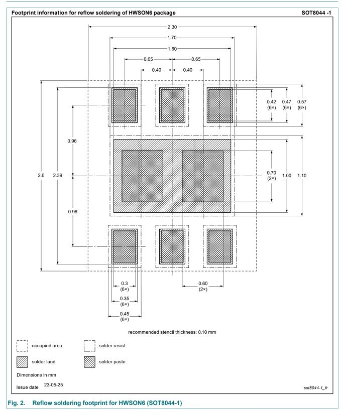
plastic thermal enhanced very very thin Small Outline packages, no leads; 6 terminals; 0.65 mm pitch; 2.0 mm x 2.0 mm x 0.75 mm body
