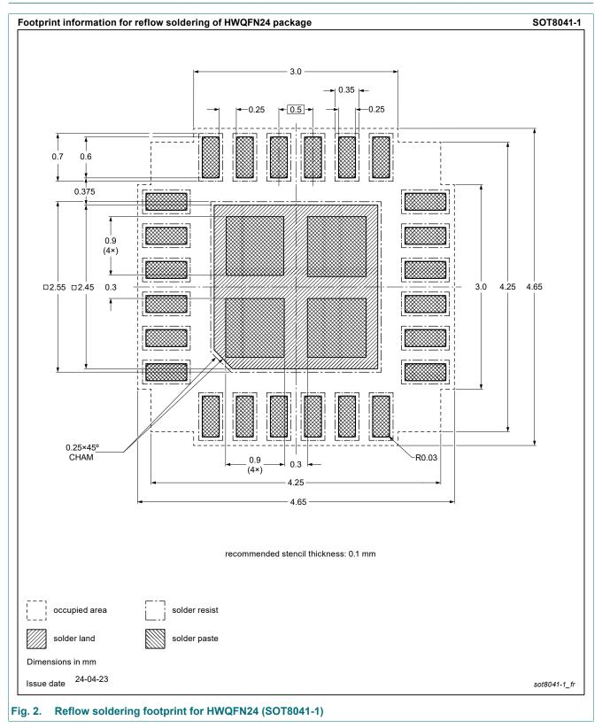
plastic thermal enhanced very very thin Quad Flat packages, no leads; 24 terminals; 0.5 mm pitch; 4 x 4 x 0.75 mm body
