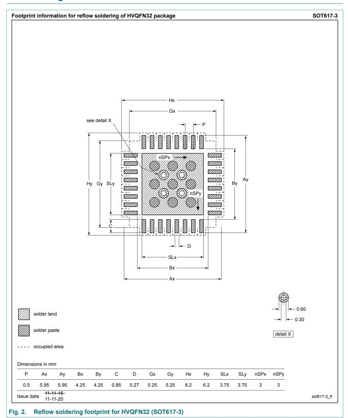
plastic, leadless thermal enhanced very thin quad flat package; 32 terminals; 0.5 mm pitch; 5 mm x 5 mm x 0.85 mm body
