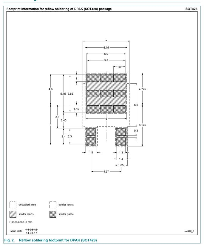
plastic, single-ended surface-mounted package (DPAK); 3 leads; 2.285 mm pitch; 6 mm x 6.6 mm x 2.3 mm body
