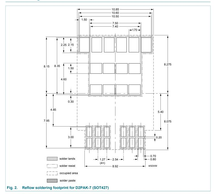
plastic, single-ended surface-mounted package (D2PAK-7); 7 leads; 1.27 mm pitch; 11 mm x 10 mm x 4.3 mm body
