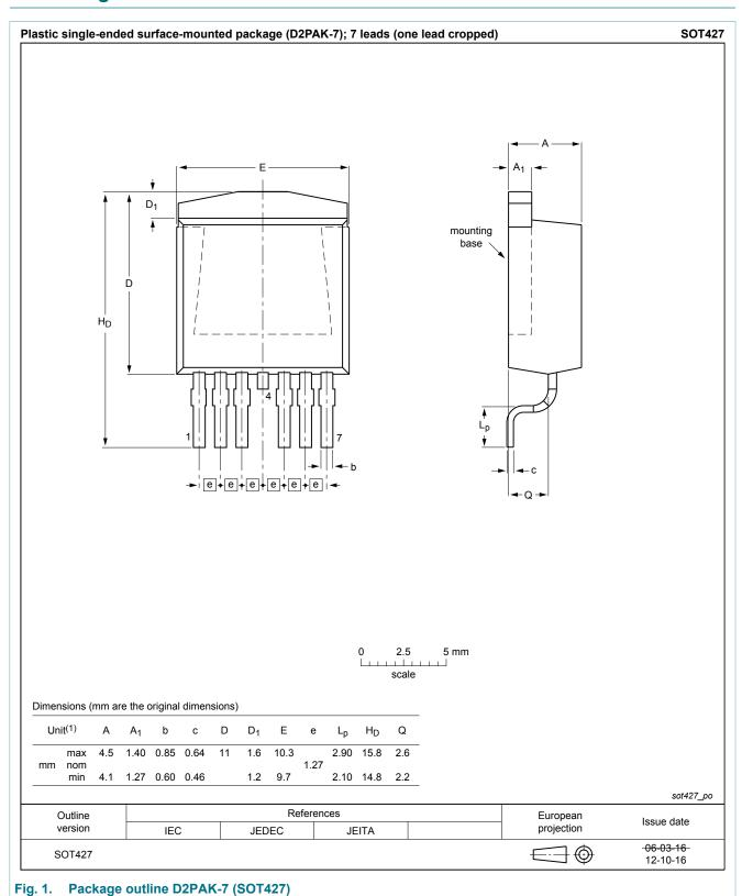
plastic, single-ended surface-mounted package (D2PAK-7); 7 leads; 1.27 mm pitch; 11 mm x 10 mm x 4.3 mm body
