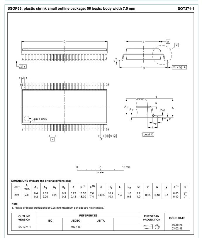
Fig. 1. Package outline SSOP56 (SOT371-1)
