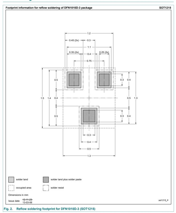
plastic, leadless thermal enhanced ultra thin small outline package with side-wettable flanks (SWF); 3 terminals; 0.75 mm pitch; 1.1 mm x 1 mm x 0.37 mm body
