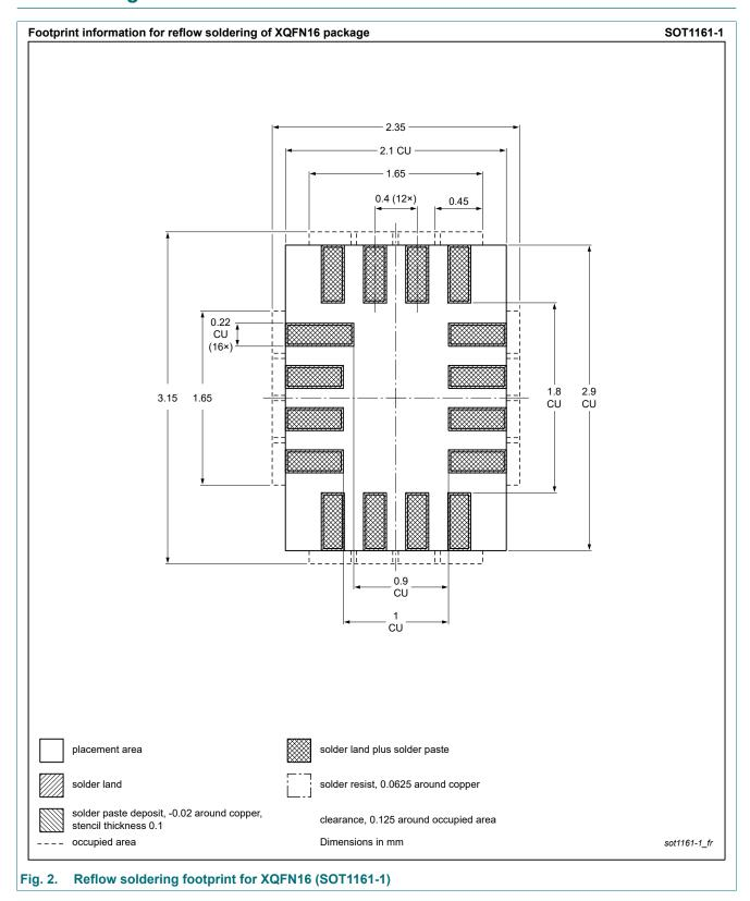
plastic, leadless extermely thin quad flat package; 16 terminals; 0.4 mm pitch; 2.6 mm x 1.8 mm x 0.5 mm body
