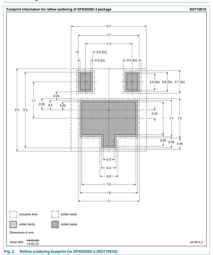
plastic, leadless thermal enhanced ultra thin small outline package with side-wettable flanks (SWF); no leads; 3 terminals; 1.3 mm pitch; 2 mm x 2 mm x 0.65 mm body
