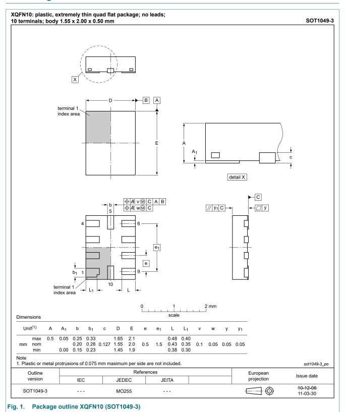
plastic, leadless extremely thin quad flat package; 10 terminals; 0.5 mm pitch; 1.55 mm x 2 mm x 0.5 mm body
