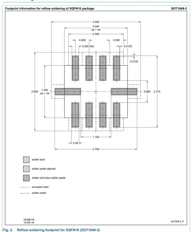
plastic, leadless extremely thin quad flat package; 10 terminals; 0.5 mm pitch; 1.55 mm x 2 mm x 0.5 mm
