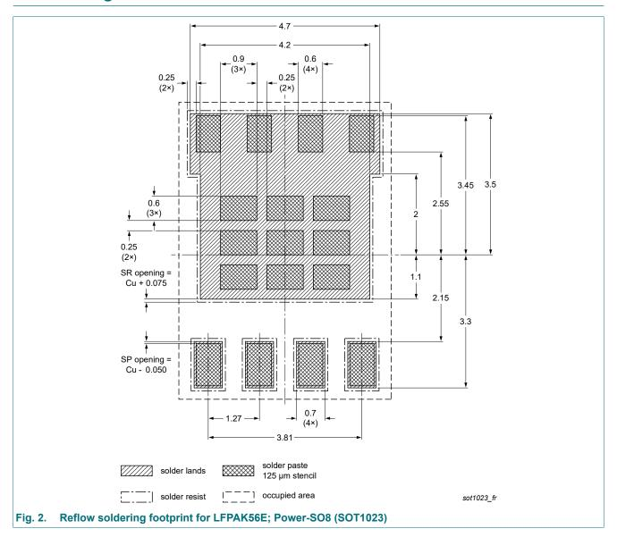
plastic, single-ended surface-mounted package (LFPAK56E); 4 leads; 1.27 mm pitch
