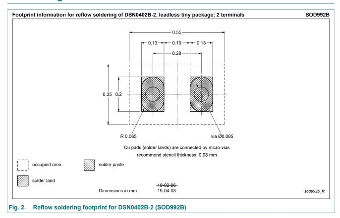
silicon, leadless tiny package; 2 terminals; 0.28 mm pitch; 0.43 mm x 0.23 mm x 0.12 mm body
