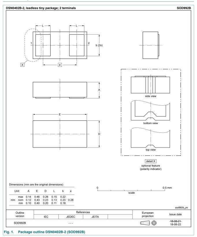
silicon, leadless tiny package; 2 terminals; 0.28 mm pitch; 0.43 mm x 0.23 mm x 0.12 mm body
