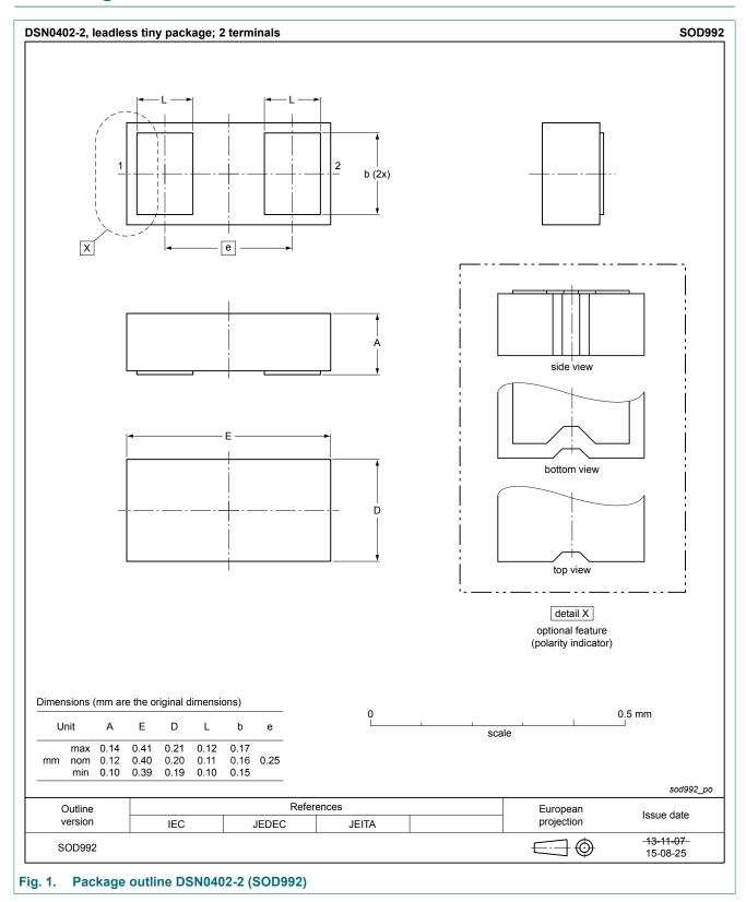
silicon, leadless tiny package; 2 terminals; 0.25 mm pitch; 0.4 mm x 0.2 mm x 0.1 mm body
