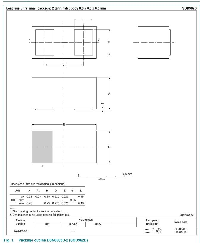
silicon, leadless ultra small package; 2 terminals; 0.36 mm pitch; 0.6 x 0.3 x 0.3 mm body
