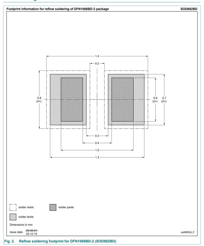
Leadless ultra small plastic package with side-wettable flanks (SWF); 2 terminals; 0.65 mm pitch; 1 mm x 0.6 mm x 0.47 mm body
