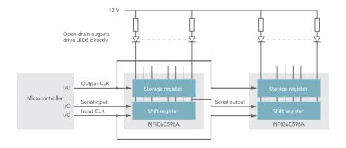
Example: drive up to 24 LEDs using just 3 controller I/Os with NPIC6C596A, substantially reducing footprint compared to using 74HC595 in combination with external MOSFETs.
