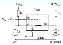
Adjust fi voltage to obtain 0 dBm level at input.
