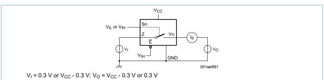
Fig. 5. Test circuit for measuring OFF-state leakage current
