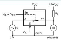
Adjust  $f_i$  voltage to obtain 0 dBm level at output. Increase  $f_i$  frequency until dB meter reads -3 dB.  $R_S = R_L = 50 \ \Omega$  (standard  $50 \ \Omega$  system).
