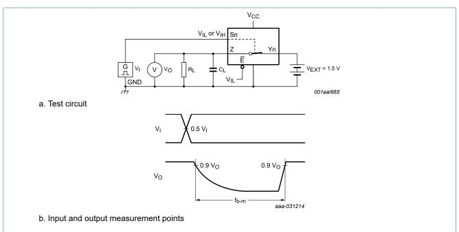
Fig. 16. Test circuit for measuring break-before-make times
