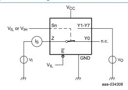
$V_I$  = 0.3 V or  $V_{CC}$  - 0.3 V;  $V_O$  =  $V_{CC}$  - 0.3 V or 0.3 V
