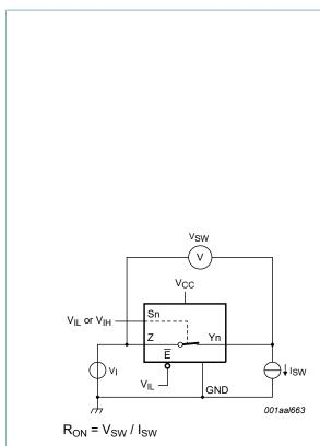
Fig. 7. Test circuit for measuring ON resistance
