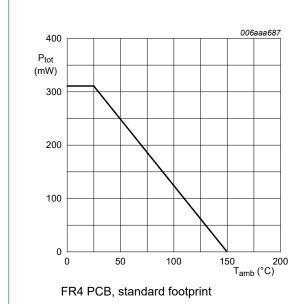
Fig. 4. Power derating curve
