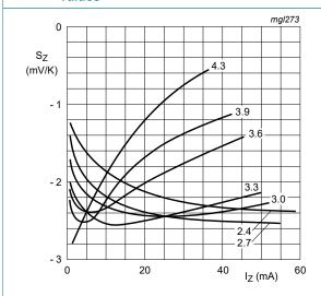
$T_i$  = 25 °C to 150 °C  $V_Z = 2.4 \text{ V to } 4.3 \text{ V}$
