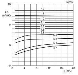
$T_i$  = 25 °C to 150 °C  $V_Z = 4.7 \text{ V to } 12 \text{ V}$
