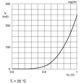
Forward current as a function of forward Fig. 2. voltage; typical values
