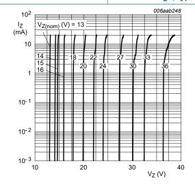
$T_j = 25 \,^{\circ}\text{C}$  $V_Z = 13 \,^{\circ}\text{V}$  to 36 V
