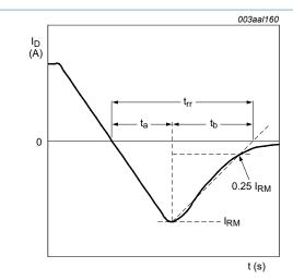
Fig. 3. Reverse recovery timing definition
