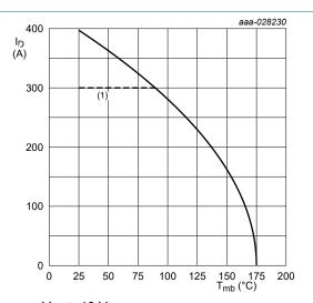
$V_{GS} \ge 10 \text{ V}$  (1) 300A continuous current has been successfully demonstrated during application tests. Practically the current will be limited by PCB, thermal design and operating temperature.
