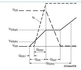
Fig. 13. Gate charge waveform definitions
