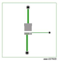
70 µm thick copper on FR4 board
