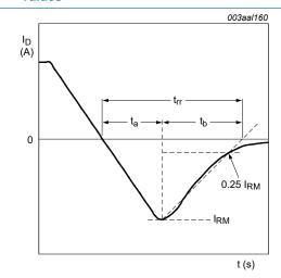
Fig. 16. Reverse recovery timing definition
