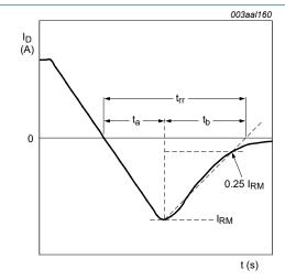
Fig. 16. Reverse recovery timing definition
