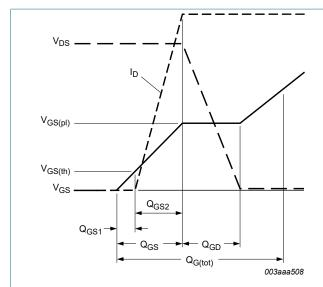
Fig. 13. Gate charge waveform definitions
