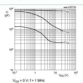
Fig. 14. Input, output and reverse transfer capacitances
