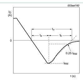
Fig. 3. Reverse recovery timing definition
