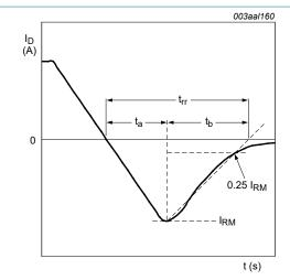
Fig. 3. Reverse recovery timing definition
