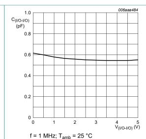
Fig. 3. Input/output to input/output capacitance as a function of input/output to input/output voltage;
