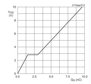
$I_D = 6 \text{ A}; V_{DS} = 10 \text{ V}; T_{amb} = 25 \text{ °C}$
