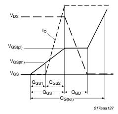
Fig 15. Gate charge waveform definitions
