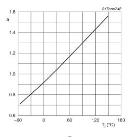
$a = \frac{R_{DSon}}{R_{DSon(25^{\circ}C)}}$
