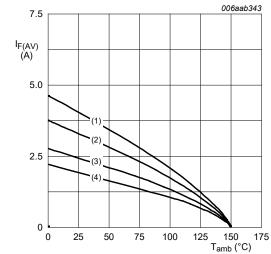
FR4 PCB, mounting pad for cathode 1 cm<sup>2</sup> T<sub>i</sub> = 150 °C
