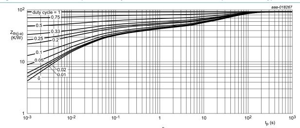
FR4 PCB, mounting pad for anode and cathode 1 cm<sup>2</sup> each
