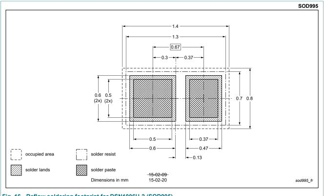
Fig. 16. Reflow soldering footprint for DSN1006U-2 (SOD995)
