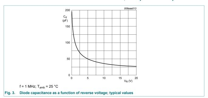
20 V, 2 A very low VF Schottky barrier rectifier
