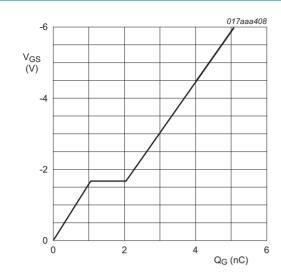
$I_D = -3.3 \text{ A}; V_{DS} = -10 \text{ V}; T_{amb} = 25 ^{\circ}\text{C}$
