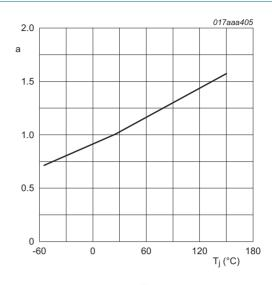
$a = \frac{R_{DSon}}{R_{DSon(25^{\circ}C)}}$
