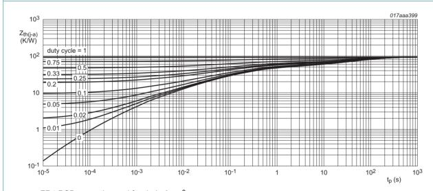
FR4 PCB, mounting pad for drain 6 cm<sup>2</sup>
