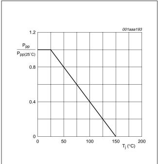
Fig.5 Relative variation of peak pulse power as a function of junction temperature; typical values.
