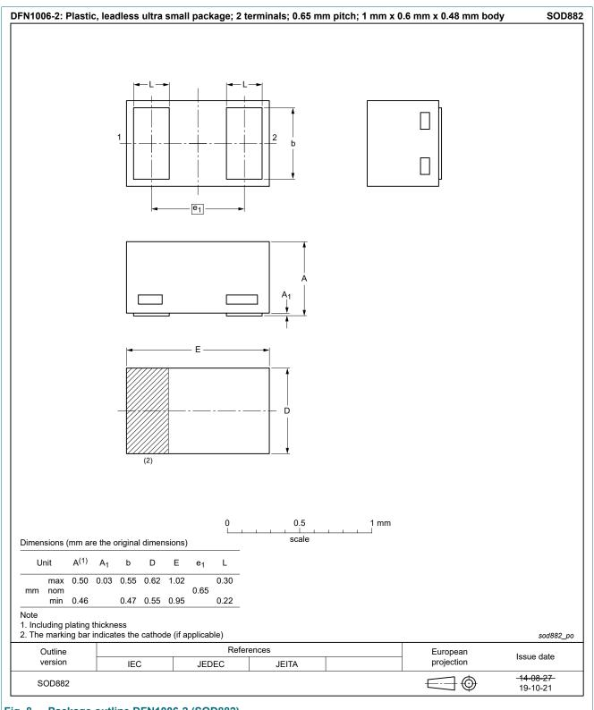
Fig. 8. Package outline DFN1006-2 (SOD882)
