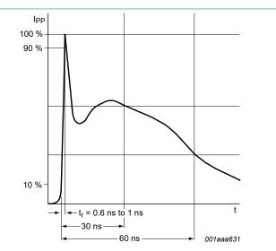
Fig. 2. ESD pulse waveform according to IEC 61000-4-2
