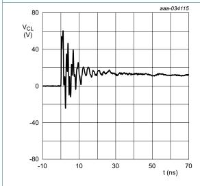
Fig. 5. Clamped +8 kV ESD pulse waveform (IEC 61000-4-2 network)
