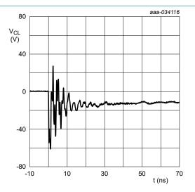
Fig. 6. Clamped -8 kV ESD pulse waveform (IEC 61000-4-2 network)
