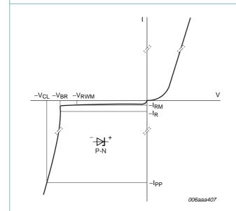
Fig 5. V-I characteristics for a unidirectional ESD protection diode
