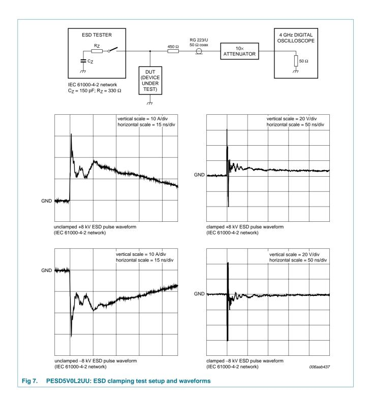
Low capacitance unidirectional ESD protection diodes
