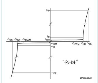
Fig 6. V-I characteristics for a bidirectional ESD protection diode
