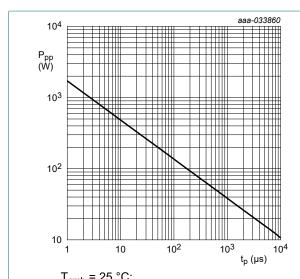
$T_{amb}$  = 25 °C;  $t_p$  = 8/20 µs exponential decay waveform
