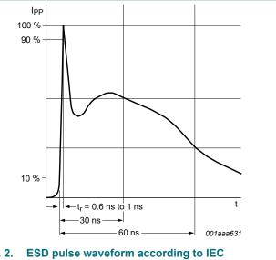
Fig. 2. ESD pulse waveform according to 61000-4-2
