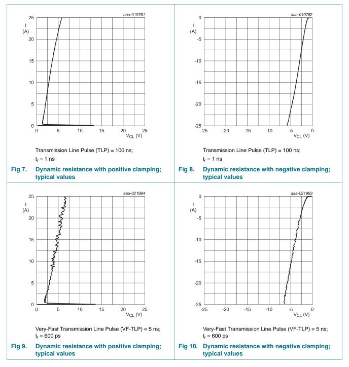
The device uses an advanced clamping structure showing a negative dynamic resistance. This snapback behavior strongly reduces the clamping voltage to the system behind the ESD protection during an ESD event. Do not connect unlimited DC current sources to the data lines to avoid keeping the ESD protection device in snapback state after exceeding breakdown voltage (due to an ESD pulse for instance).
