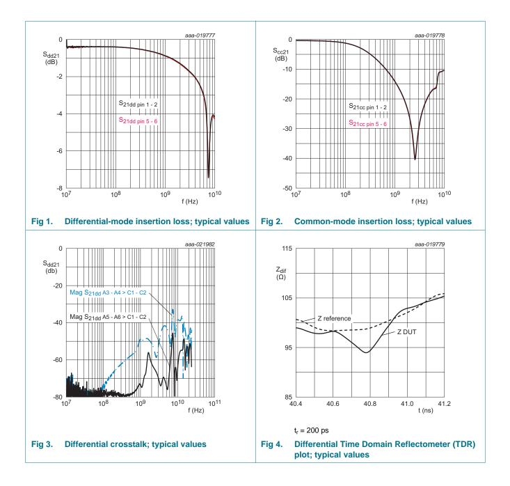
Common-mode EMI filter for differential channels with ESD protection
