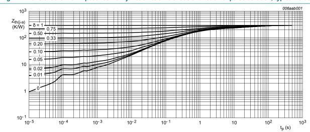
FR4 PCB, single-sided, 35 µm copper, tin-plated, mounting pad for collector 1 cm<sup>2</sup>.
