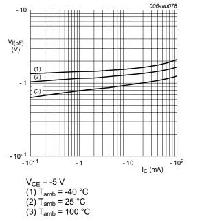
g. 9. Off-state input voltage as a function of collector current; typical values
