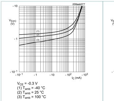
Fig. 8. On-state input voltage as a function of collector current; typical values
