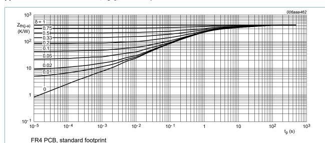
Fig. 2. TR1 (PNP): Transient thermal impedance from junction to ambient as a function of pulse duration; typical values
