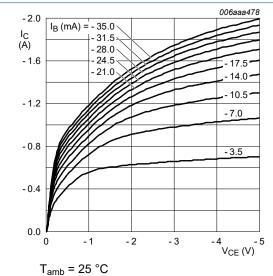
Fig. 9. TR1 (PNP): Collector current as a function of collector-emitter voltage; typical values
