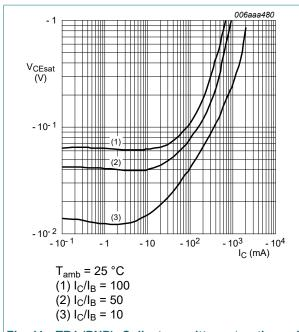
Fig. 11. TR1 (PNP): Collector-emitter saturation voltage as a function of collector current; typical values
