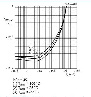
Fig. 6. TR1 (PNP): Collector-emitter saturation voltage as a function of collector current; typical values
