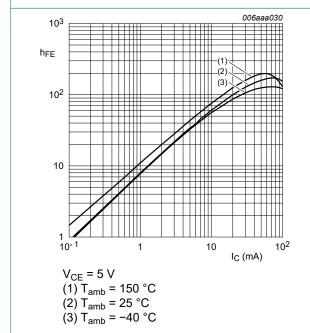
Fig. 13. TR2 (NPN): DC current gain as a function of collector current; typical values
