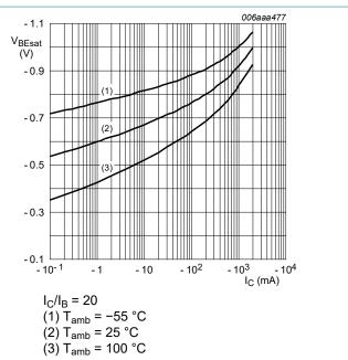
Fig. 8. TR1 (PNP): Base-emitter saturation voltage as a function of collector current; typical values
