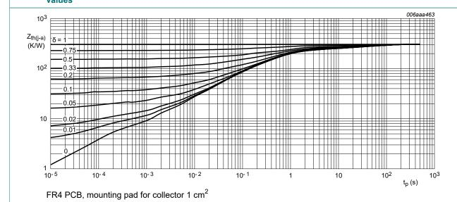
Fig. 3. TR1 (PNP): Transient thermal impedance from junction to ambient as a function of pulse duration; typical values
