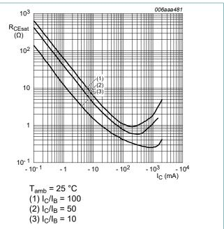
Fig. 12. TR1 (PNP): Collector-emitter saturation resistance as a function of collector current; typical values
