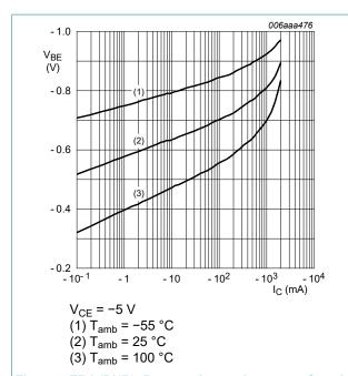
Fig. 7. TR1 (PNP): Base-emitter voltage as a function of collector current; typical values
