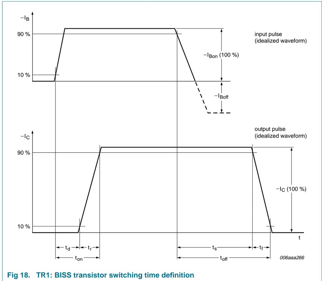
Fig 18. TR1: BISS transistor switching time definition
