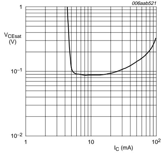
$I_C/I_B = 50; T_{amb} = 25\text{ °C}$
