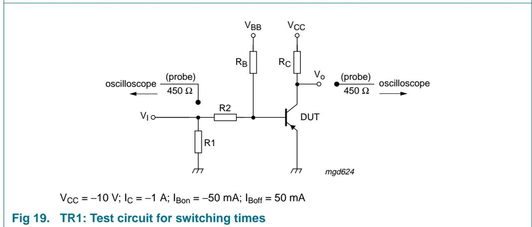
Fig 19. TR1: Test circuit for switching times
