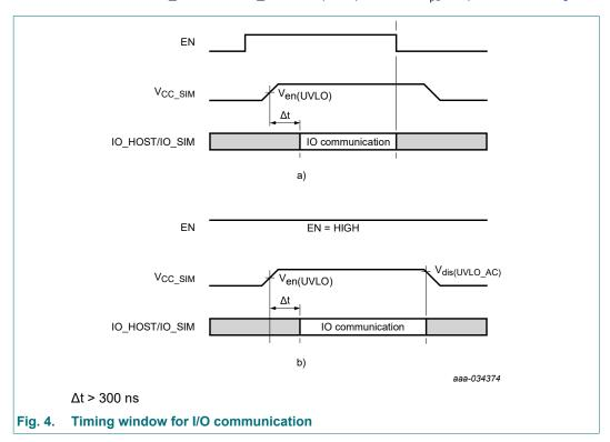
When either EN turns low or  $V_{CC\_SIM}$  drops below  $V_{dis(UVLO)}$ , the translator turns to shutdown mode. Section 8.3 illustrates the shutdown sequence in more detail.
