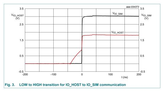
Looking at the input signal, the first part of the LOW to HIGH transition is an exponential curve caused by the I/O node capacitance being charged via the pull-up resistor. The second part starts when the input signal crosses the input switching level. The rising edge is accelerated dramatically by the PMOST that is turned on by the one shot on the input side.
