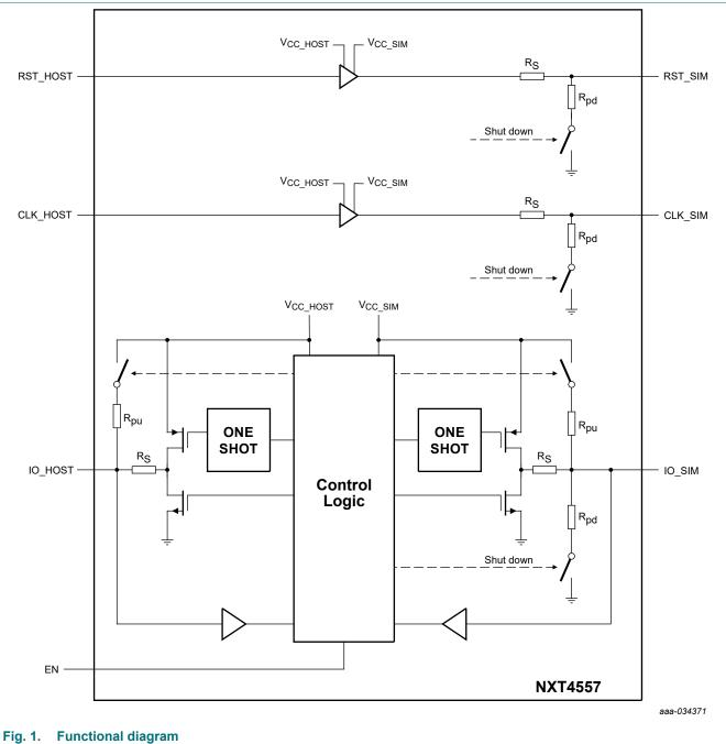
SIM card interface level translator with enable pin
