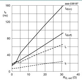
$V_{DD}$  = 800 V;  $I_{D}$  = 40 A;  $V_{GS}$  = -5/15 V; L = 82  $\mu$ H;  $T_{i}$  = 25 °C
