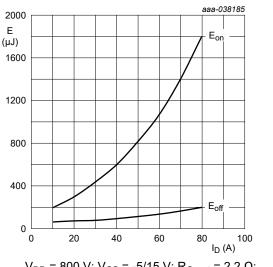
$V_{DD}$  = 800 V;  $V_{GS}$  = -5/15 V;  $R_{G,\;ext}$  = 2.2  $\Omega;$  L = 82  $\mu H;\; T_i$  = 25 °C
