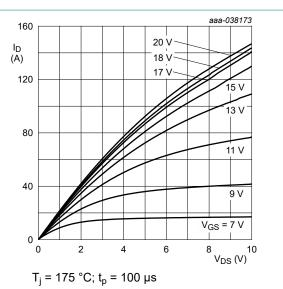
Fig. 2. Output characteristics: drain current as a function of drain-source voltage; typical values
