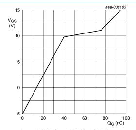
$V_{DD} = 800 \text{ V}; I_D = 40 \text{ A}; T_j = 25 ^{\circ}\text{C}$
