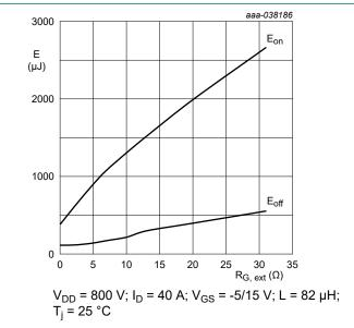
Fig. 15. Switching loss as a function of external gate resistance; typical values
