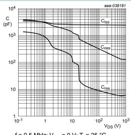
$f = 0.5 \text{ MHz}; V_{GS} = 0 \text{ V}; T_j = 25 \text{ °C}$
