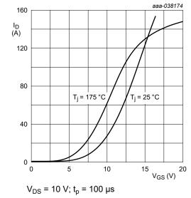
Fig. 3. Transfer characteristics: drain current as a function of gate-source voltage; typical values
