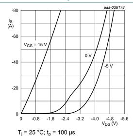
Fig. 7. Source current as a function of sourcedrain voltage; typical values (third quadrant characteristics)
