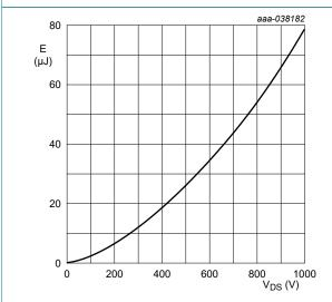
Fig. 11. C<sub>oss</sub> stored energy as a function of drain-souce voltage; typical values
