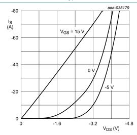
$T_j$  = 175 °C;  $t_p$  = 100  $\mu s$ Source current as a function o
