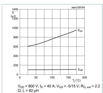
Fig. 13. Switching loss as a function of junction temperature; typical values
