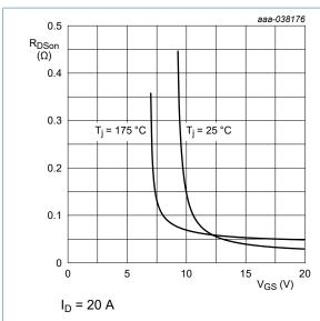
Fig. 5. Drain-source on-state resistance as a function of threshold voltage
