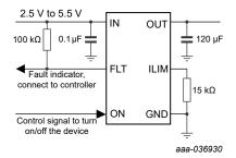
**Note:** Connect at least 120  $\mu$ F capacitor at output for USB port application, other applications except USB choose output capacitor according to actual transient requirements.
