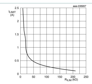
$V_{IN}$  = 5 V;  $T_{amb}$  = 25 °C
