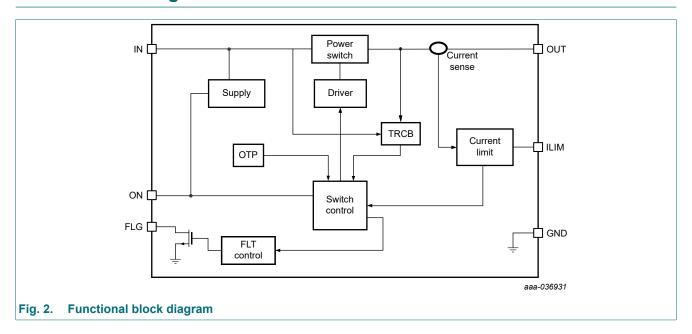
5.5 V, 55 m $\Omega$  load switch with precision adjustable current limit
